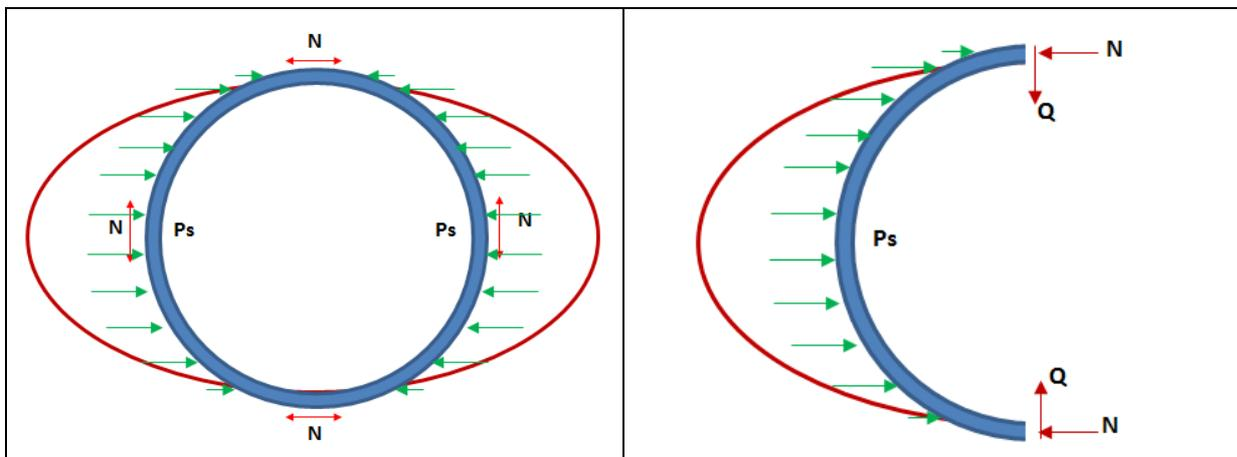
**Figure 7. Design of the shotcrete layer in flexion**
