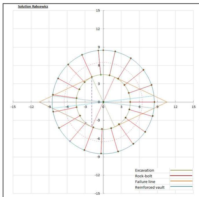
Figure 2. Failure lines and reinforced crown
