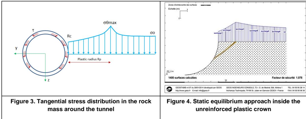
**Figure 3. Tangential stress distribution in the rock mass around the tunnel**
