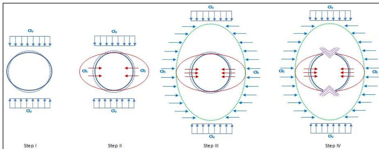
**Figure 1. Evolution of the failure mechanism of a non supported excavation, the given example is for  $sh/sv < 1.0$**
