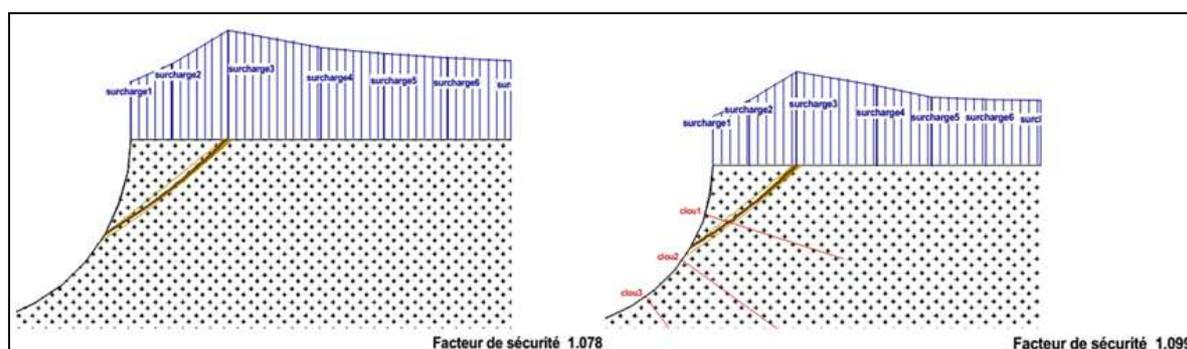
Figure 5. Global stability of a non reinforced and a rock-bolted section away from the tunnel head, GEOSTAB ©
