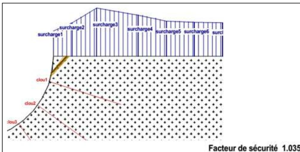
Figure 6. Local stability of the section between the rock-bolts, GEOSTAB ©
